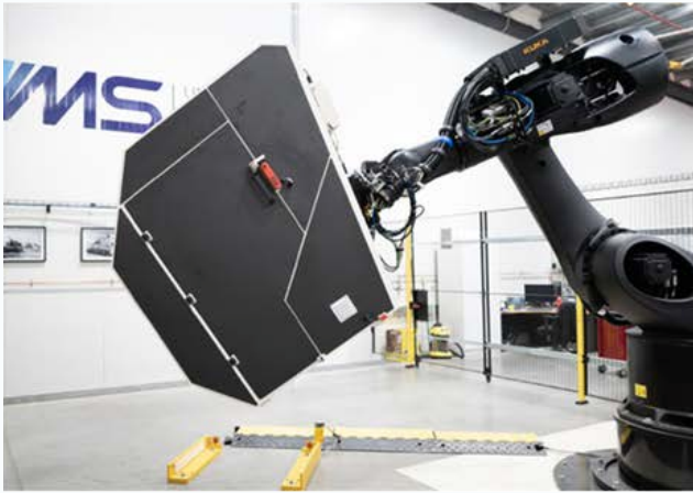
Large pitch rotation plus heave with RDS
